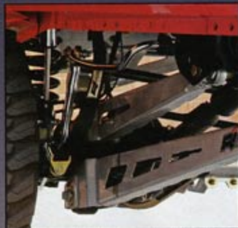
The Rize quad-link system has fully adjusted radius arms.
