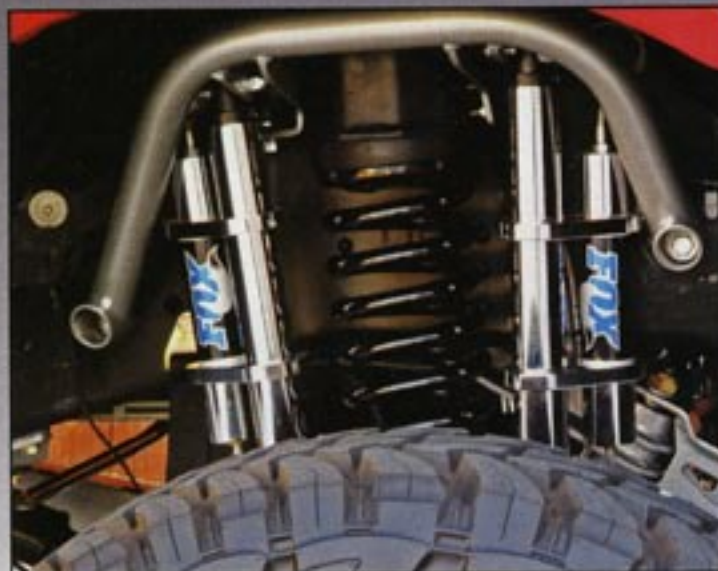
Fox shocks and a Fabtech dual-shock hoop combine at the front for a smooth ride.
