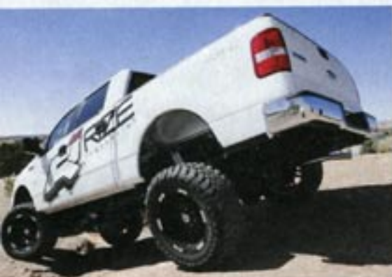
▲ The tail section is lifted with a pair of blocks and is damped using high-quality Bilstein 5150 shocks.
