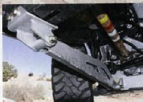
▲ Radius-arm-style impact struts mean that the drop cradle is effectively braced. This is part of the reason we're calling this kit an upgrade. Without the impact struts, the drop cradle would place heavy leverage on the frame at the cradle mounting points and we'd have to call this kit a modification instead.
