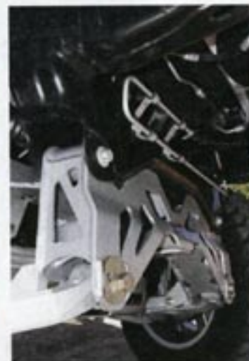
◀ The entire system is based on laser-cut, 1/4-inch, CNC-formed steel that's cut, formed, and welded in house. Systems are available in silver or black powdercoat.
