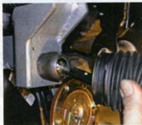
▲ Rize Industries found advantages in dropping the steering linkage to meet the OEM tie rod locations on the knuckles. The advantages are a lighter steering feel and reduced stress on the steering rack. The Rize linkage uses unique brackets to get the job done. First, the steering bracket bolts to the rack in place of the OEM tie rods. The rack remains bolted in its stock location. The steering bracket moves back and forth smoothly and steadily thanks to three sealed cam follower bearings. Finally, the stock tie rods bolt between the Rize linkage and the Rize knuckle.
