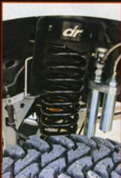
Up front are a dual-steering stabilizer that uses performance shocks and 2-1/2-inch spring spacers.
