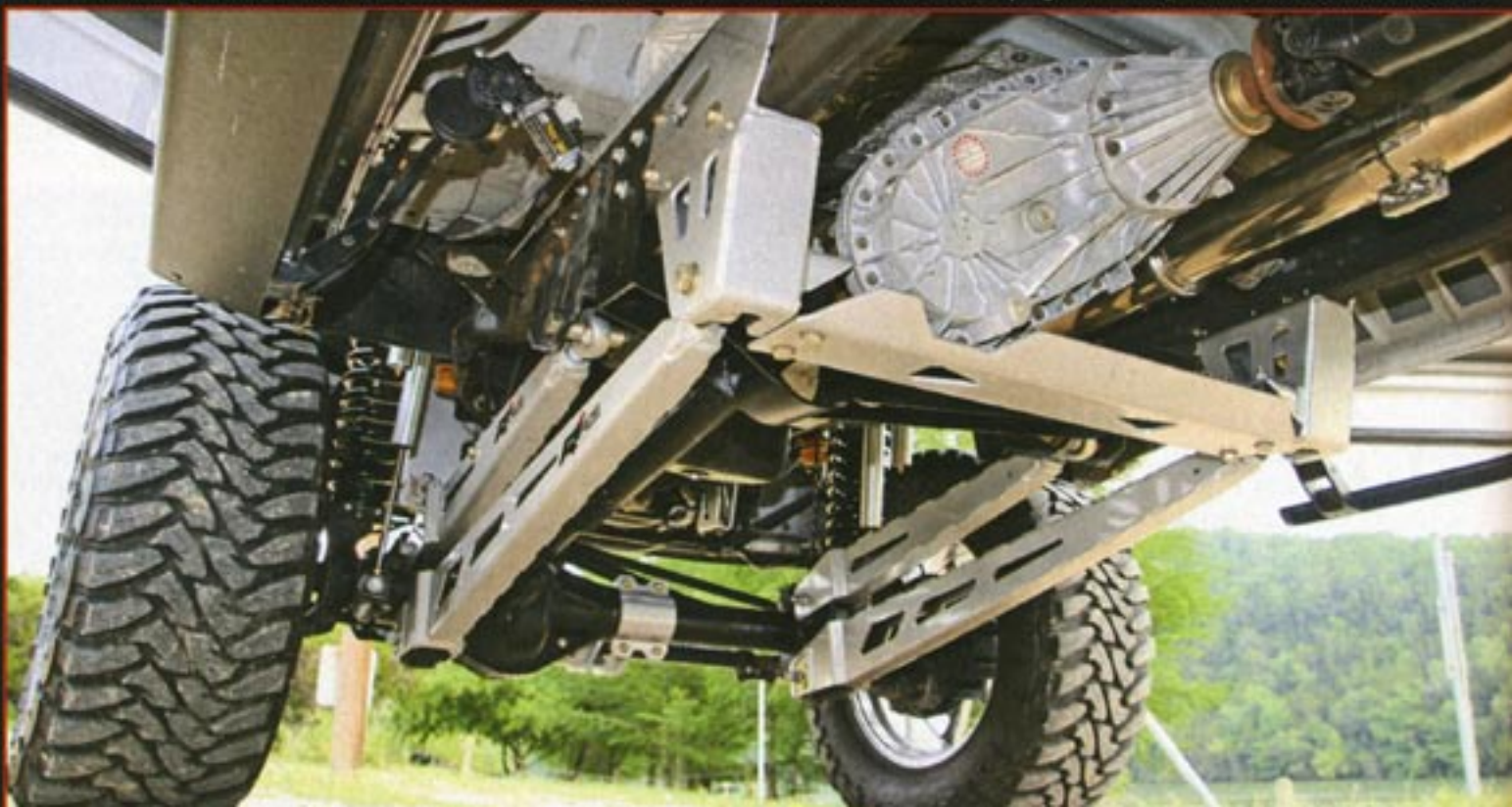
An 8-inch lift kit using Rize's trick four-link kit. The rear has floating traction bars and dual shock kits, and soft-ride springs and shocks, and there is a custom CV driveshaft.
