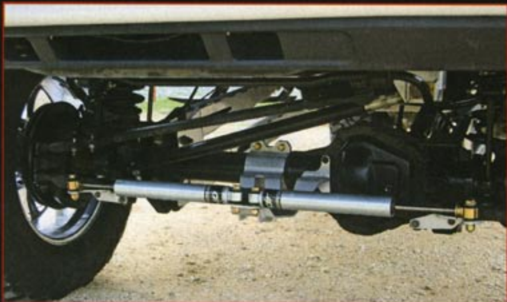
An 8-inch lift kit using Rize's trick four-link kit. The rear has floating traction bars and dual shock kits, and soft-ride springs and shocks, and there is a custom CV driveshaft.
